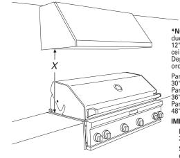
\*NOTE: The grill vent hood duct cover is designed to add 12" (30.5 cm) to meet the ceiling or soffit height.
